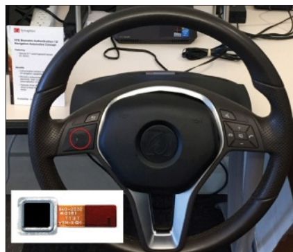
Fig. 2: In a working steering-wheel demonstration (circled in red), the capacitive fingerprint sensor (inset) also doubles as a directional pad (D-Pad) for navigating the in-car user interface.
